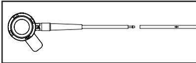
**Figure 1. Band tubing and port tubing connection**
